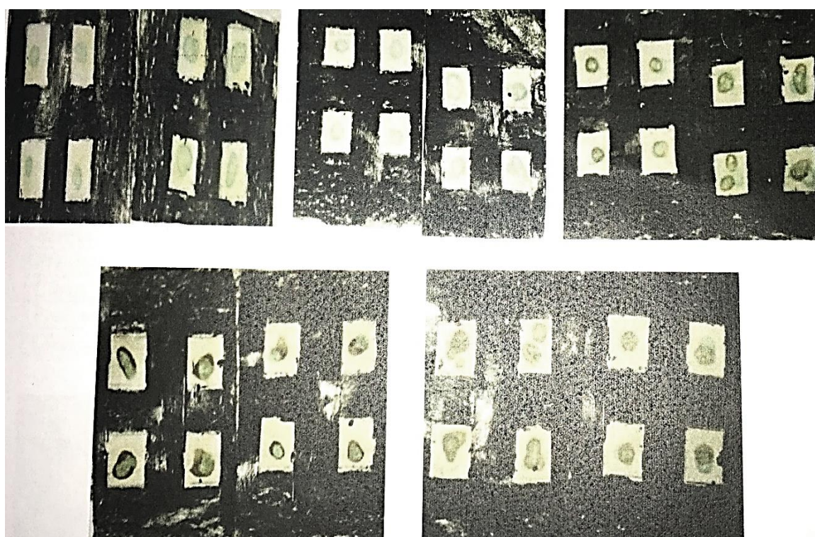
Figure 4. Alkaloid identification using paper-based colorimetric strips.
